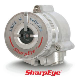
The new 40/40R Single IR Flame Detector detects hydrocarbon-based fuel and gas fires using advanced flame analysis tools. The detector provides early warning of flaming fires working at 4.5 µm for maximum sensitivity, and immunity to false alarms from IR sources such as sunlight and IR projectors.
