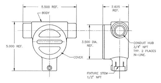
Figure 7. Optional Explosion Proof Mounting Box, P/N 06-116317-001
